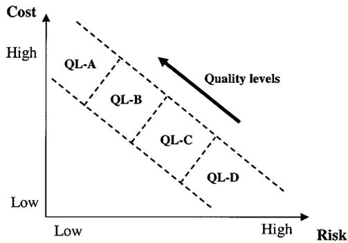
Fig. 1. Quality levels in subsurface utility engineering
